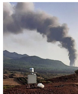
Figure 1. Sampler collecting PM 10 samples in La Palma during the 2021 volcanic eruption.
