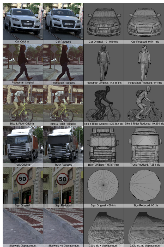
Fig. 3 We illustrate the impact of polygon count reduction on specific classes and how a reduced polygon count may affect visual quality (left). We also show wireframe visualizations (on the right) showing the changes in the overall geometric shape due to polygon reduction. Note that the displacement used is a per-pixel process that tessellates the geometry on demand during the rendering process, to create a more complex geometry
