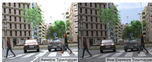
Fig. 8 In the absence of a proper tonemapping algorithm, higher luminance values are typically compressed, exhibiting overexposed image regions (left). Contrary, using better tonemapping algorithms may unveil new details in the image (right)
