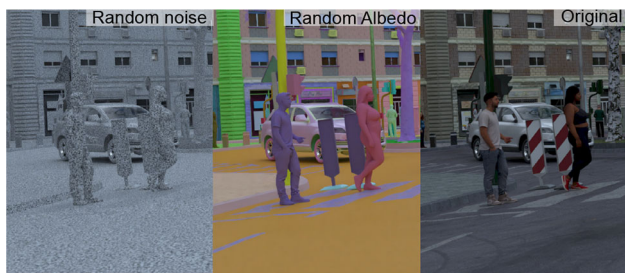
Fig. 4 UrbanSyn dataset rendered with three material modeling approaches tested in our experiments: (left) using a procedurally generated random noise to replace the albedo; (center) using random solid colors facilitating object parts differentiation; and (right) UrbanSyn’s original approach with realistic BRDF and textures
