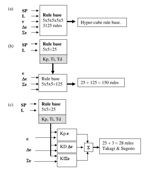
Fig. 1. Some strategies in reducing Rule bases. (a), Original hyper-cube rule base. (b), Two rule bases in series. (c), Reduction based on Takagi & Sugeno method.
