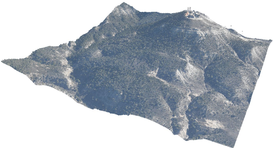
Fig. 8 One of the misclassified mountain tiles, classified as forest, shown using the RGB data of each point
