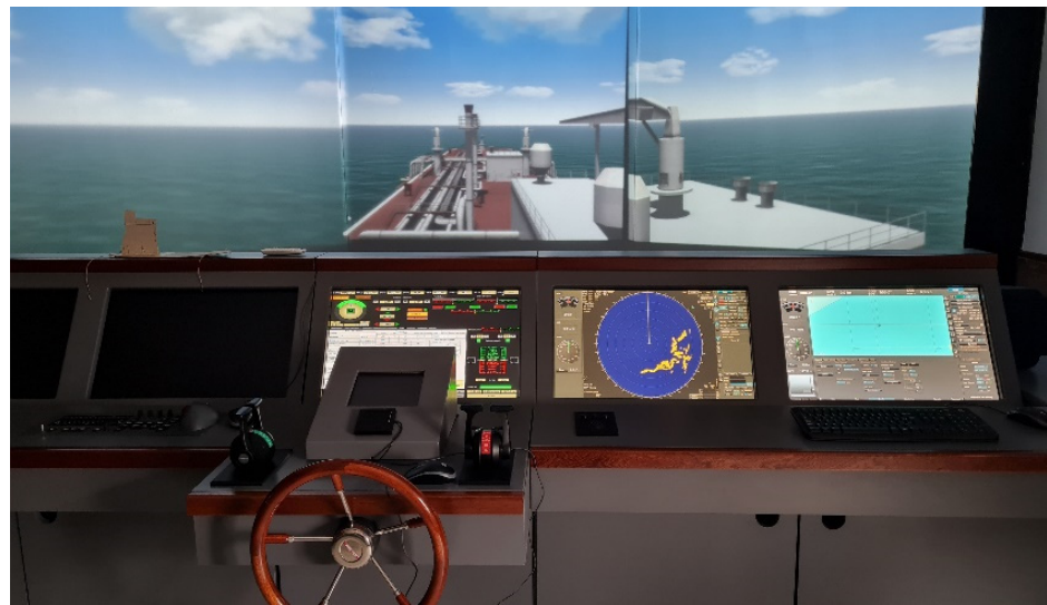
Figure 1. Vision of the full mission simulator with the steering instruments and some bridge equipment.
