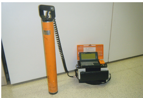
FIGURE 1: Picture of the portable gamma-ray spectrometer GF Instruments model GRS-2000 used for field measurements in this work. On the left side, the probe with the detector can be seen, and on the right side, the computer system with electric supply can be seen.
