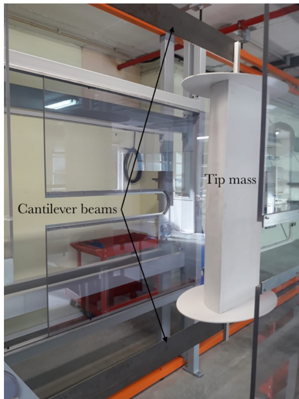
Figure 8: Energy harvesting prototype mounted in the test chamber.
