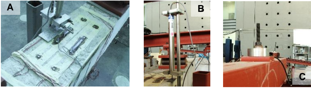
Fig. 7 Test instrumentation. A: Strain gauges on concrete beams. B: Displacement transducer. C: Load cell
