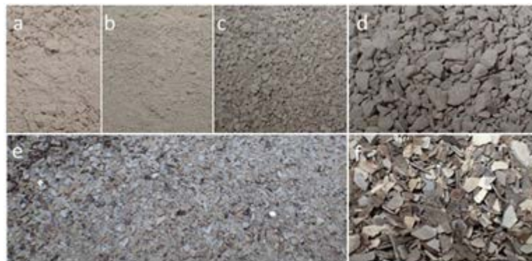
Fig. 1. Sand aggregates: a) Limestone sand 0-0.063mm b) Limestone sand 0.063-0.25 mm c) Limestone sand 0.25-1mm d) Limestone sand 1-4mm e) Fine mussel shell sand (FMS) 0-1mm f) Coarse mussel shell sand (CMS) 0-4mm
