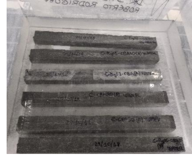
Fig. 6: Specimens immersed in water
