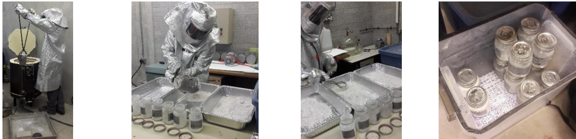
Fig. 3: MEA obtaining process: taking out from the kiln, pouring and spreading on trays and packing.
