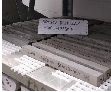
Fig. 5: Specimens in air-drying conditions
