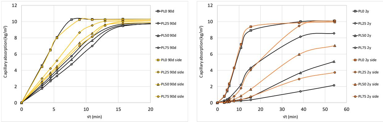
Figure 8. Capillary curves in samples placed parallel and perpendicular to cast direction, at 90 days age (left), 2 years (right).
