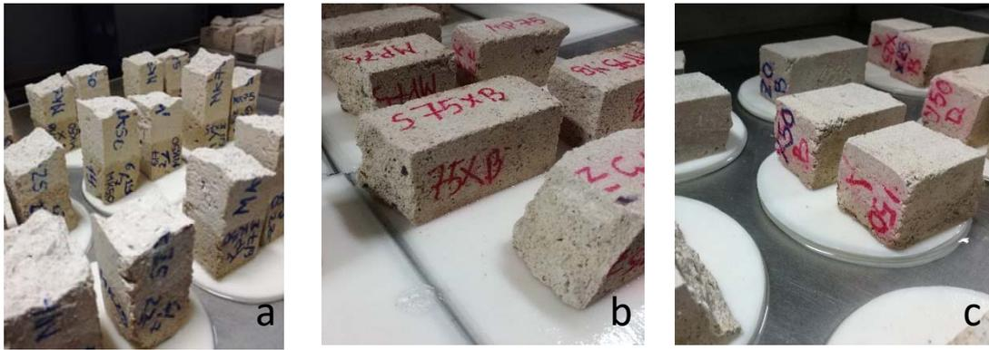
Figure 1. Capillary test: a) standard test, b) specially designed test – parallel to cast direction, c) specially designed test – perpendicular to cast direction.
