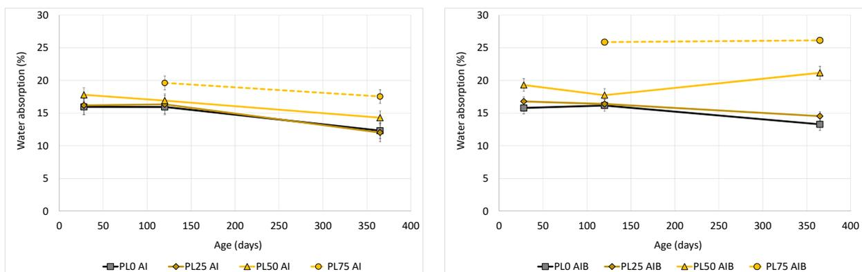
Figure 3. Water absorption at 28 days, 120 days and 1 year.
