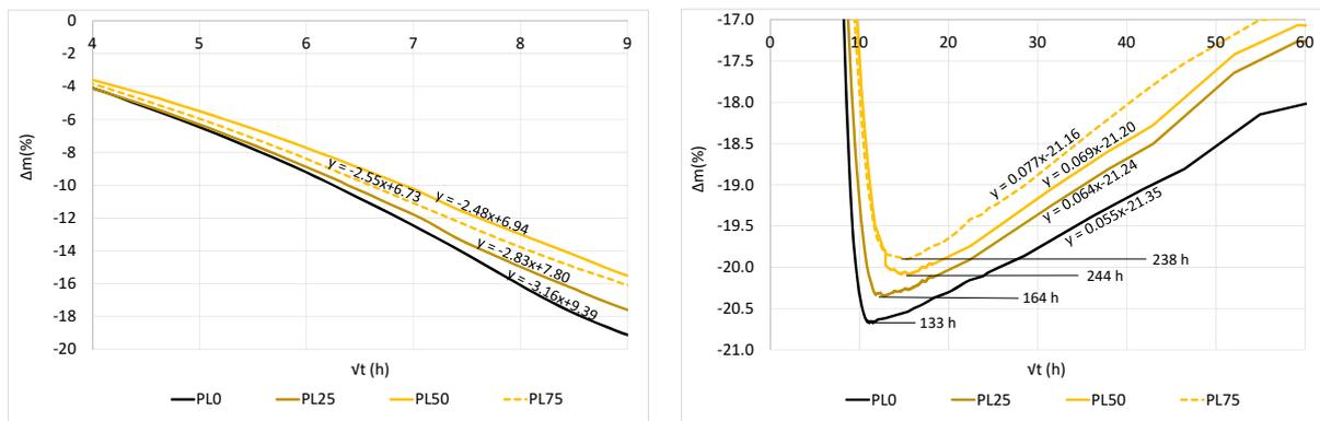
Figure 10. Details of the two predominant stages in weight variation from fresh state: water evaporation stage (left) and carbonation stage (right).
