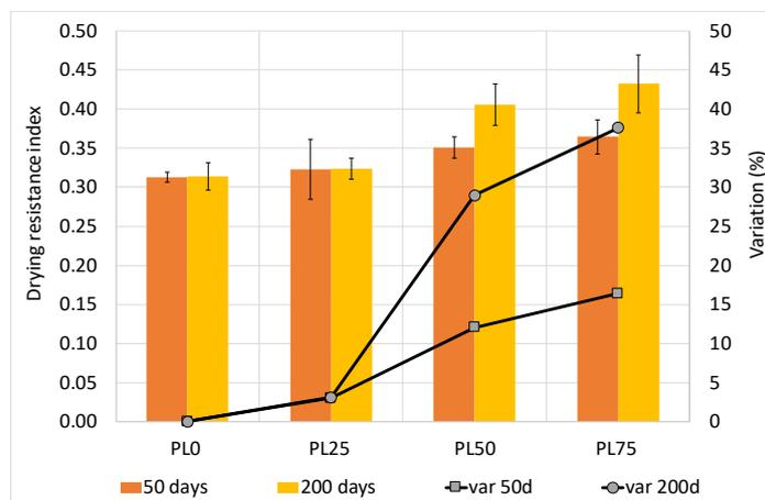
Figure 12. Drying resistance index of lime mortars at 50 and 200 days.
