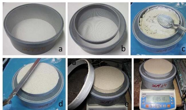
Figure 2. Drying test in fresh state: a) plastic mesh, b) PVC tube, c) casting, d) levelling, e) demoulding, f) weighing.
