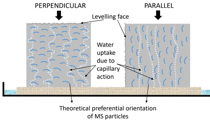
Figure 7. Water uptake test. Perpendicular to cast direction (left) and parallel to cast direction (right).
