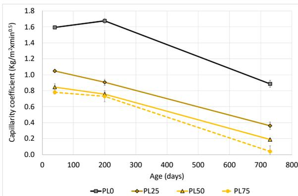
Figure 5. Capillary coefficient at 40 days, 200 days, and 2 years.
