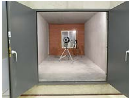
Figure 14. Reverberation room to carry out sound reduction tests.
