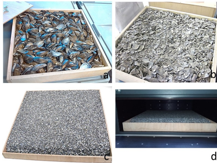
Figure 11. Boxes for thermal test: a) entire shell, b) mussel shell gravel, c) coarse mussel shell sand, d) box in the heat flow meter device.
