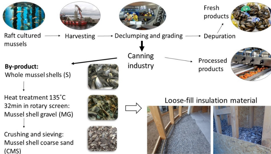
Figure 1. Process to obtain mussel shell insulation material.
