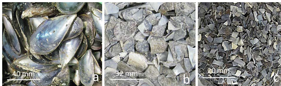
Figure 2. Mussel shell used: a) whole mussel shell (S), b) mussel shell gravel (MG), c) coarse mussel shell sand (CMS).
