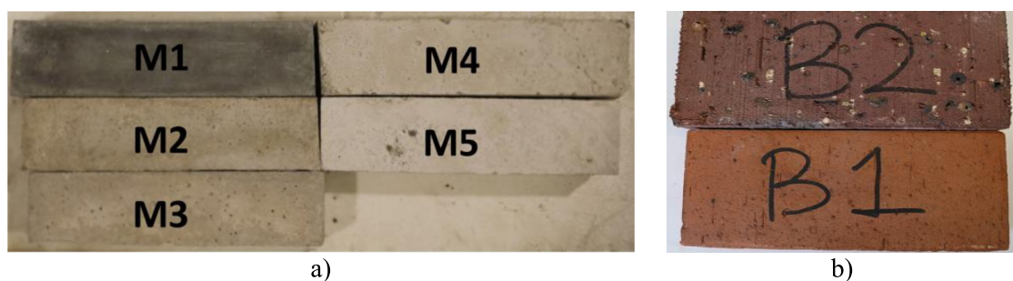
Figure 1. Constituents of Masonry Prism a) Masonry mortar b) Prismatic bricks.
