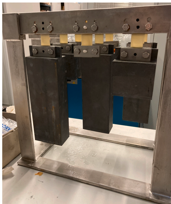
Fig. 3. Second rack outside the container, used to hold the upper crossbars with samples during gravimetric analysis.
