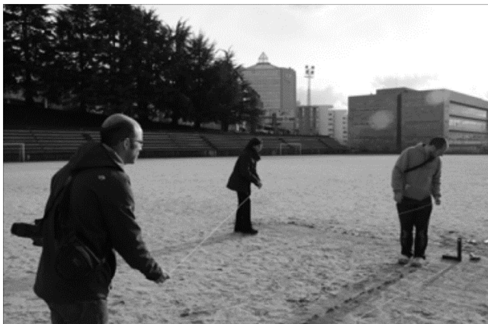
Figure 4 Realization of the initial stakeout using the Pythagorean triangle. Experiment carried out at the football pitch of the University of Santiago de Compostela on March 21, 2017. © Ruben Vuelta-Santín
