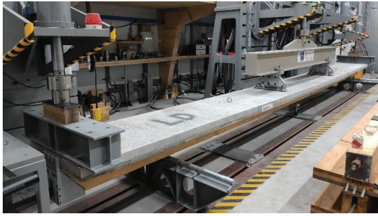
Figure 12: Type A test arrangement, with cantilevers at the end of the beam.
