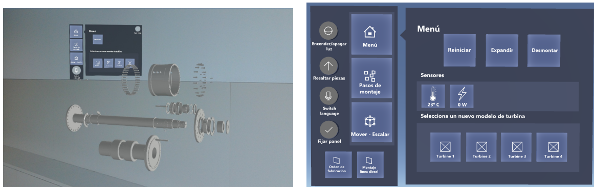
Figure 8. 3D model of the clutch after the disassembly animation (left) and a screenshot of the control panel (right).
