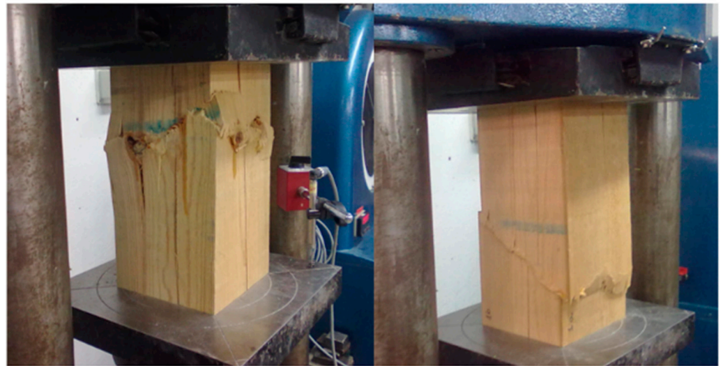
Figure 2. Image of the compression testing of an unreinforced piece of wood.
