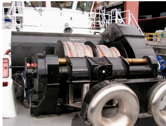
Figure 11. Asymmetric Render/Recover ® Hawser Electric Winch model DESDF-48-200 from Markey Machinery.
