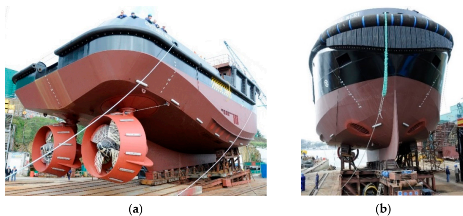
Figure 3. (a,b) The ASD escort tug “Costante Neri” delivered in September 2009 by Gondán Shipyard, S.A. (Spain), to the owner Fratelli Neri S.p.A. (Italy). Photo: Authors.
