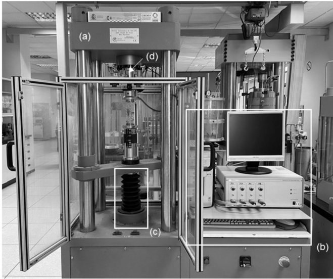
Fig. 3. General view of the testing equipment: (a) Testing frame, (b) Control unit and gauge meter, (c) Double-action loading piston, and (d) Loading cell.
