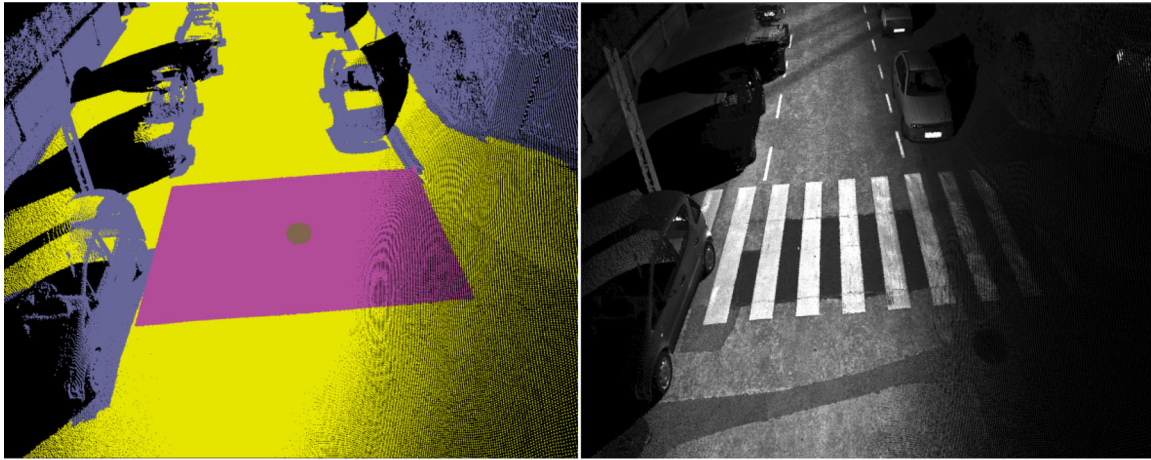
(a) Zebra crossing with obstacles in point cloud view
