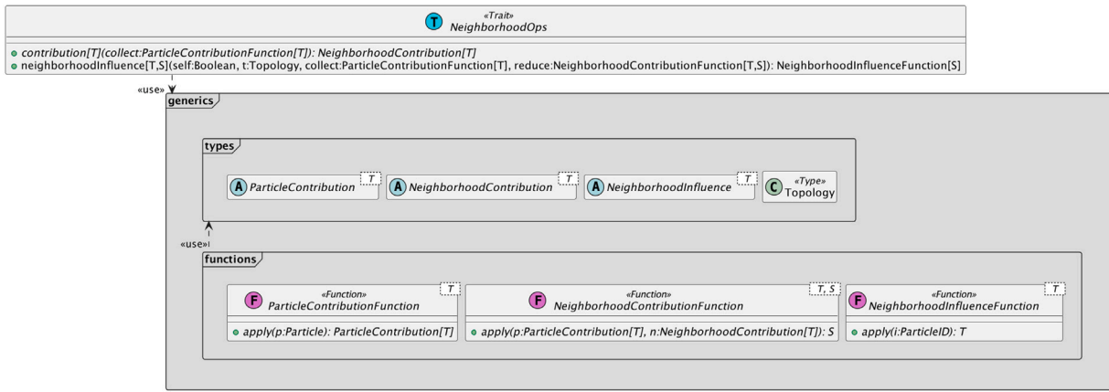
Fig. 12. Class diagram of the generic types and functions to represent models of influence.
