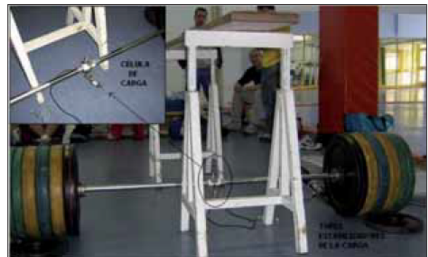
Figure 2 - Placement of the chain in the load cell
