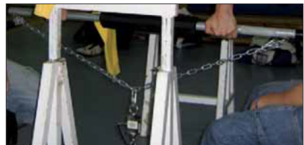
Figure 2 - Placement of the chain in the load cell
