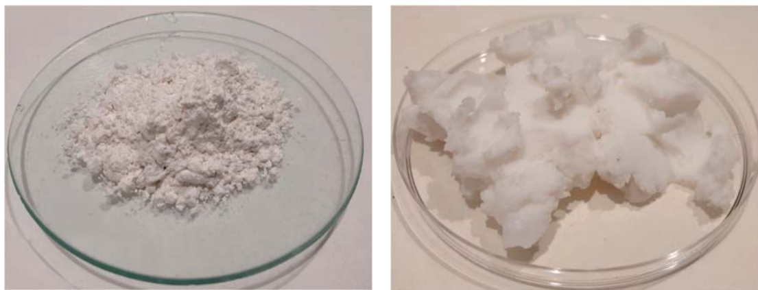
Figure 2. Two types of nanocellulose used in the present research: a) CNC and b) CNF.
