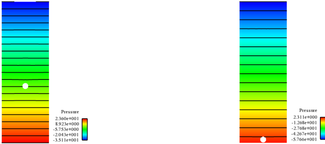
FIG. 7.7. 2D Motion of a cylinder: isopressure contours for \eta = 0.1 and \rho^s = 1.25 at t = 14.295 and t = 41.99 , respectively, and for \Delta t = 0.02 .
