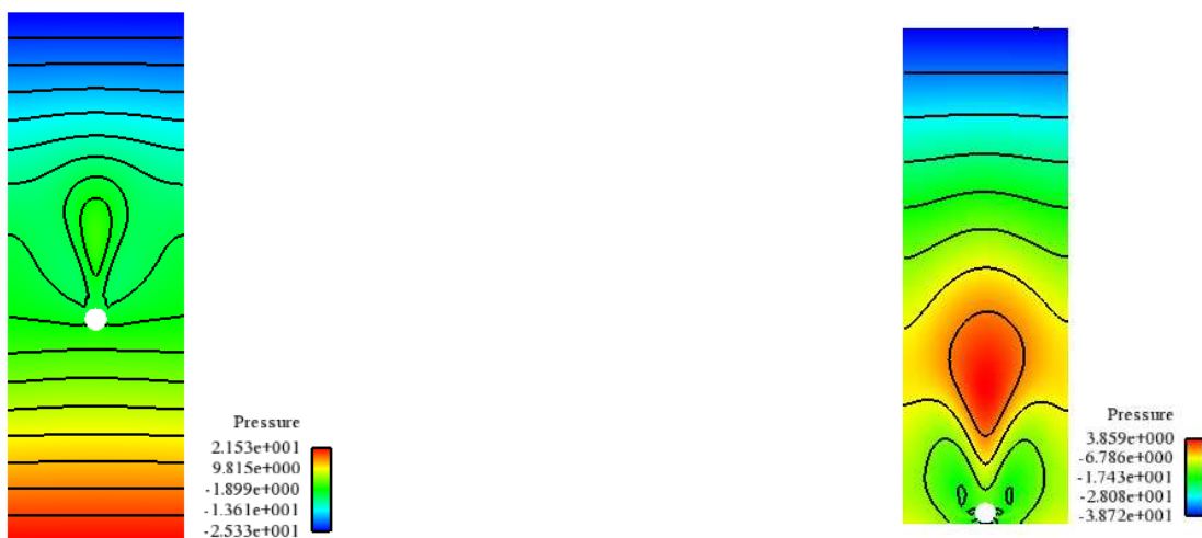
FIG. 7.9. 2D Motion of a cylinder: isopressure contours for \eta = 0.01 and \rho^s = 1.5 at t = 2.2495 and t = 5.4895 , respectively, and for \Delta t = 0.001 .
