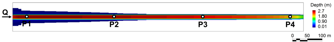
Figure 2. Example of water depth map predicted by the 2D-SWE in the synthetic case study. Location of control points (P1-P4).
