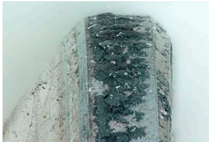
Figure 2. Accumulation of combustion waste in the check valves.
