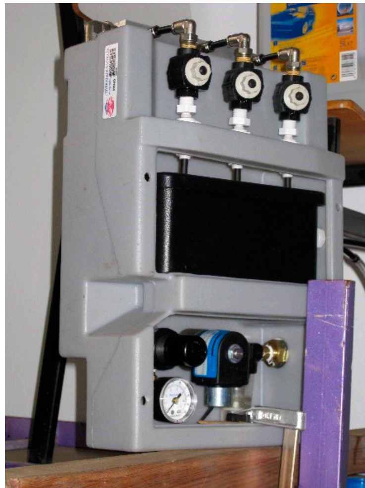
Figure 10. Adiabatic saturator (Spraying Systems Spain S.L. model 45,500).
