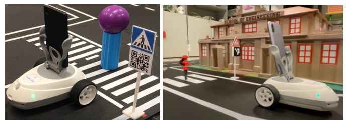
Fig. 16. Left: The “pedestrian” detected by secondary school students. Right: The pedestrian-like doll used for high-school students
