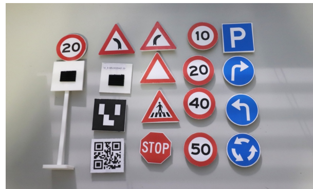
Fig. 5. Vertical traffic signs designed for the model
