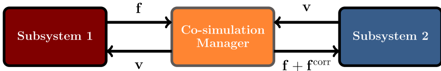
Fig. 6 Energy correction via modification of the coupling variables
