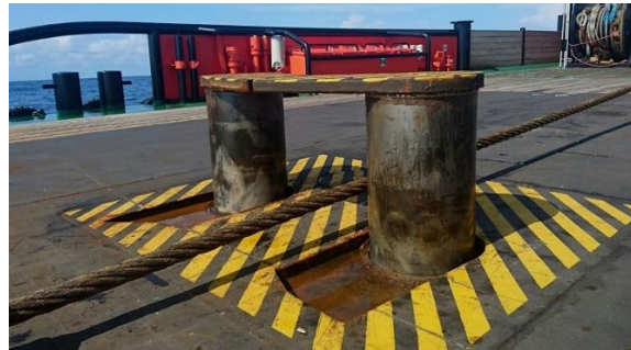
Figura 1.4.3 e 1.4.4 : Rodillo de popa e Pins de Guía dun AHTS ( Stern Rollers | PALFINGER MARINE, no date )( Towing pins - Damen Marine Components, no date )
