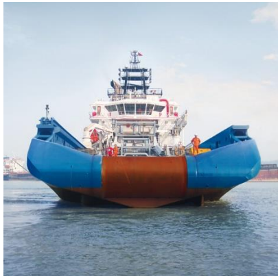
Figura 1.4.3 e 1.4.4 : Rodillo de popa e Pins de Guía dun AHTS ( Stern Rollers | PALFINGER MARINE, no date )( Towing pins - Damen Marine Components, no date )
