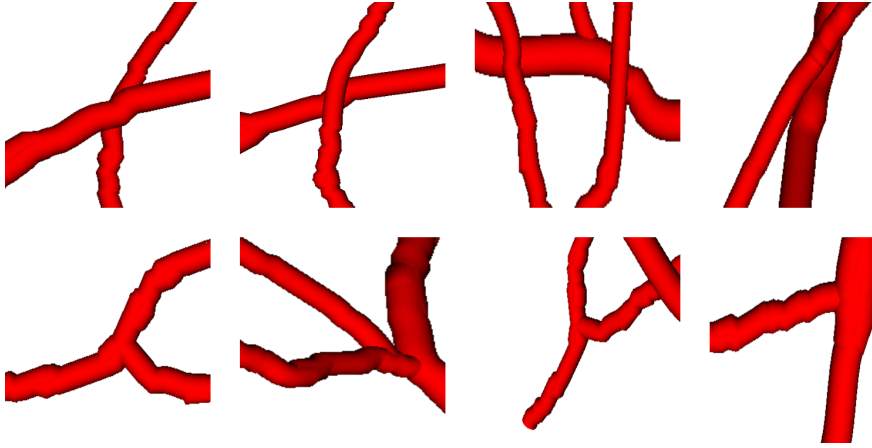
Fig. 15 3D visualization of intersections correctly managed. Row 1: examples of crossings. Row 2: examples of intersections.
