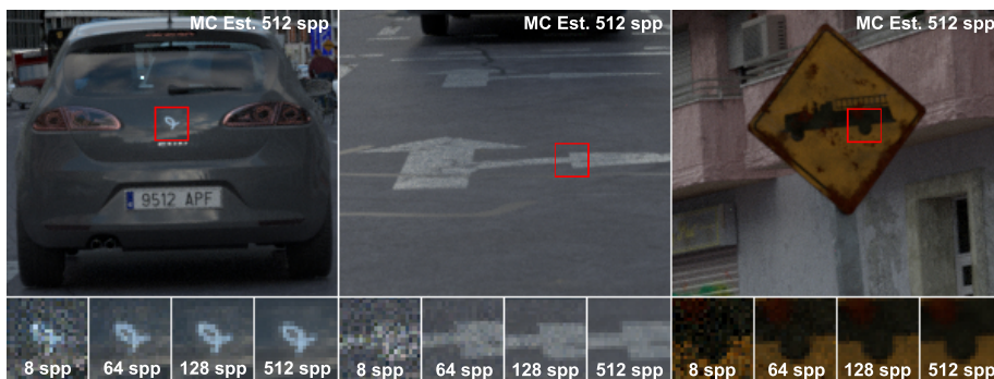
Figure 2: Various levels of Monte Carlo noise introduced by path tracing rendering. We compare how different samples per pixel could impact the semantic segmentation task.
