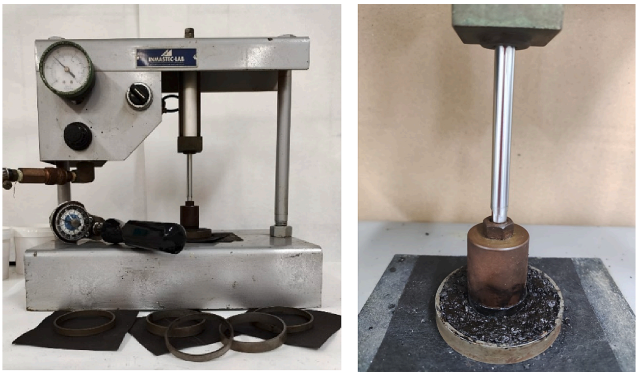
Fig. 7. Cohesion test: a) Cohesimeter and b) Torque measurement of a sample of MICROF 8.
