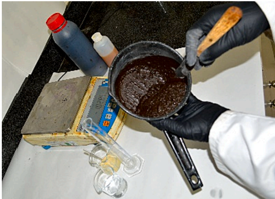
Fig. 4. MICROF 8 manufacture at laboratory scale to determine the breaking time.
