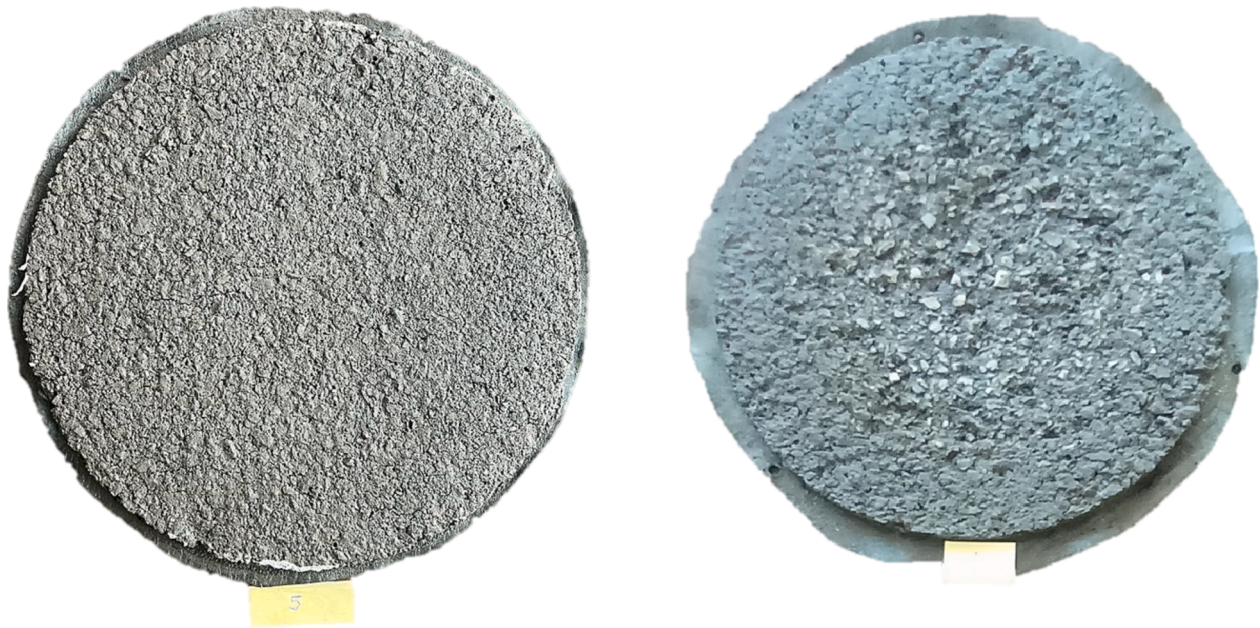
Fig. 10. Abrasion samples for MICROF 8 made with SI aggregates and 11.5% of bitumen emulsion: a) toner as mineral powder and b) cement as mineral powder.
