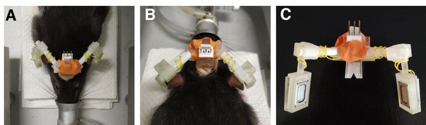
Figure 3. A , B , Front and rear view of a set of Ratphones adjusted under anesthesia. C , Set of Ratphones assembled and glued together, including the speakers, cables, and connector.
