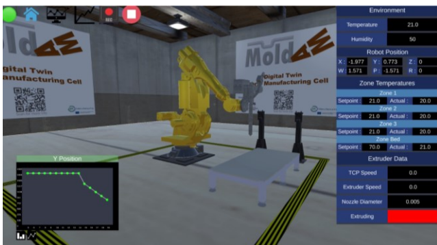
Figure 4 Screenshot of the Digital Twin generated for monitoring the behaviour of the Additive Manufacturing process
