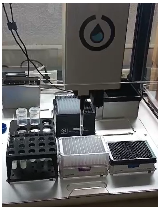
Figure 3: Opentrons OT-2 liquid-handling robot. The OT-2 already prepared to execute the protocol with all the labware in the right position. Pipettes used are the Multichannel P300 in the right mount, and the Single Channel P1000 in the left mount.
