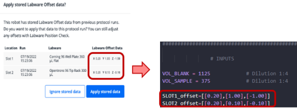
Figure 5: Using a simple protocol with the OT-2 APP allows us to get the calibration values for each SLOT.
