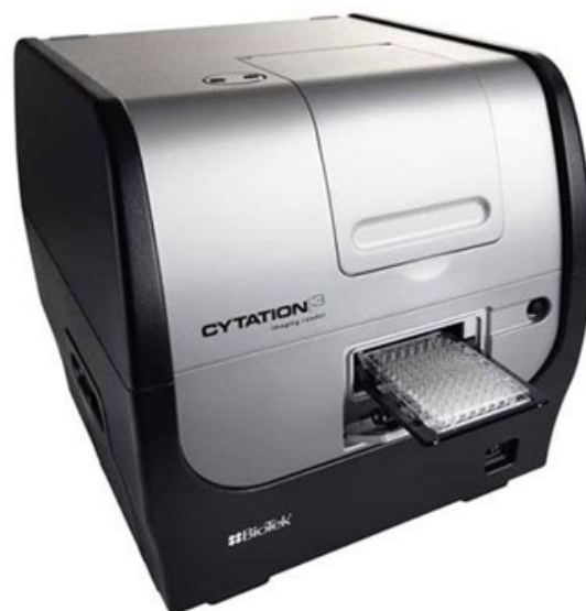
Figure 2: Agilent Biotek Cytation 3 plate reader. This plate reader allows us for incubation at 37°C, agitation and measurement of both absorbance and fluorescence.
