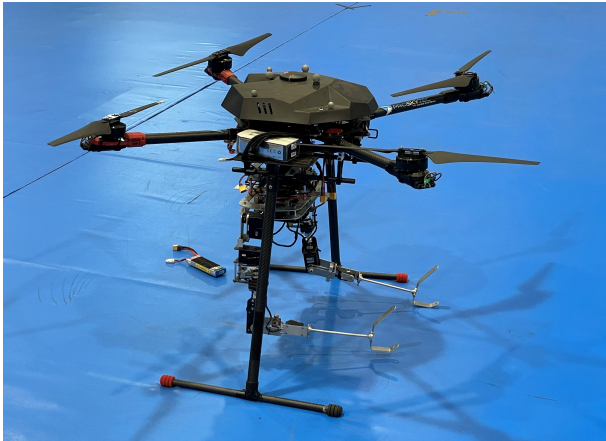
Figure 4: Multi-rotor platform integrating the LiCAS A1 dual arm manipulator used to conduct the aerial grasping of a parcel in a logistics scenario.
