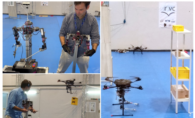
Figure 1: Experimental evaluation of the LiCAS dual arm teleoperation system with the industrial task board (left, up) and in an aerial manipulation tasks involving the grasping and delivery of a parcel (left down, right).
