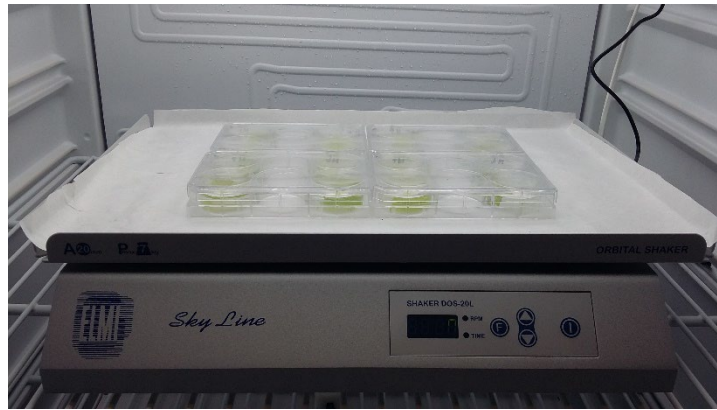
Fig. 1. Skyline shaker with Falcon® plates in the Liebherr® environmental simulation chamber.
