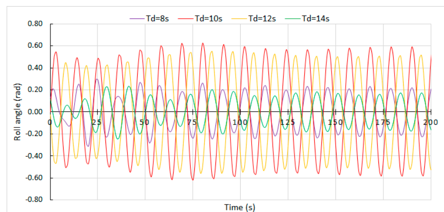
Figure 7. Rolling angles reached by different ship loading conditions for T_w = 11 s.
