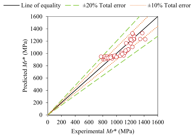
Fig. 7. Predicted versus measured characteristic resilient modulus and total error limits.
