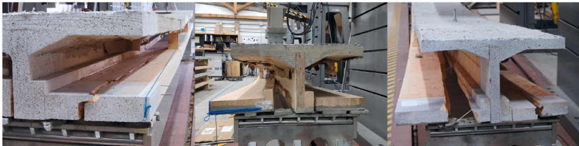
Fig. 8. Longitudinal failures of the glulam flange in tests 250.2-B, 300.1-C, and 350.1-C.
