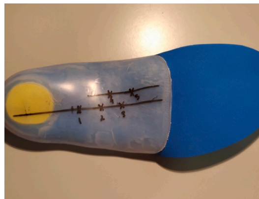
Figure 3. Orthopedic insoles manufactured for this study (crosses marked in black show the five Shore hardness measurement points).
