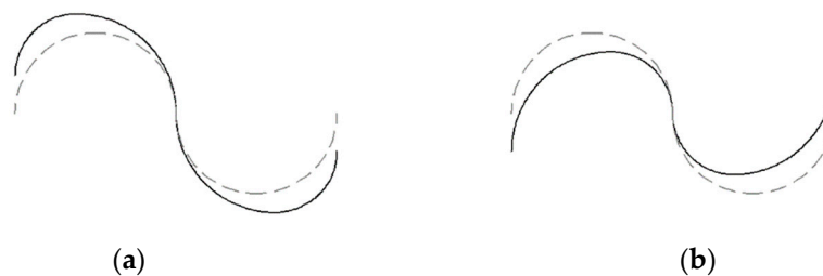
Figure 10. Blade profiles analyzed; (a) Fibonacci I (black color dashed line), sequence low-high-high-low, and comparison with Savonius (grey color dotted line); (b) Fibonacci II (black color dashed line), sequence high-low-low-high, and comparison with Savonius (grey color dotted line).
