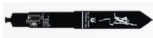
Figura 1: I2C Soil Moisture Sensor. Catnip Electronics. [6]
