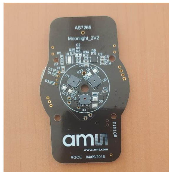
Figure 1: AS7265x board integrating three sensors able to acquire, within the spectral band ranging from 410nm to 940nm, 18 multispectral readings.
