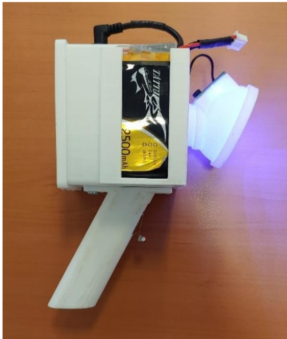
Figure 2: View of the developed 18-band low-cost and portable multispectral device, sensitive within the range 410-940nm.
