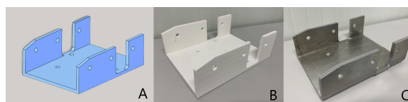
Figure 1: Evolution of the design process. A: 3D modeling, B: PLA prototype using FDM, C: final steel part.
