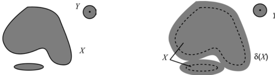
Figure 2.5: Example of Dilation working over a figure.
