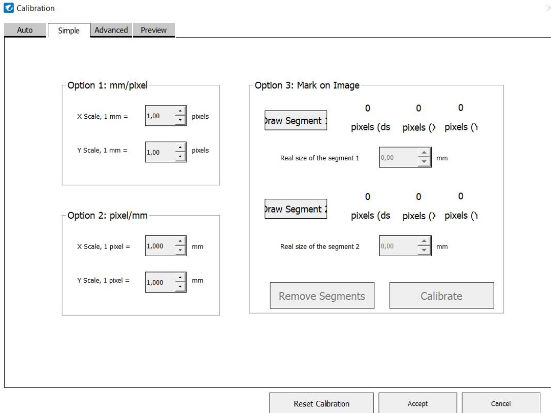
Figure 5.13: New Simple panel in the Calibration Tool.
