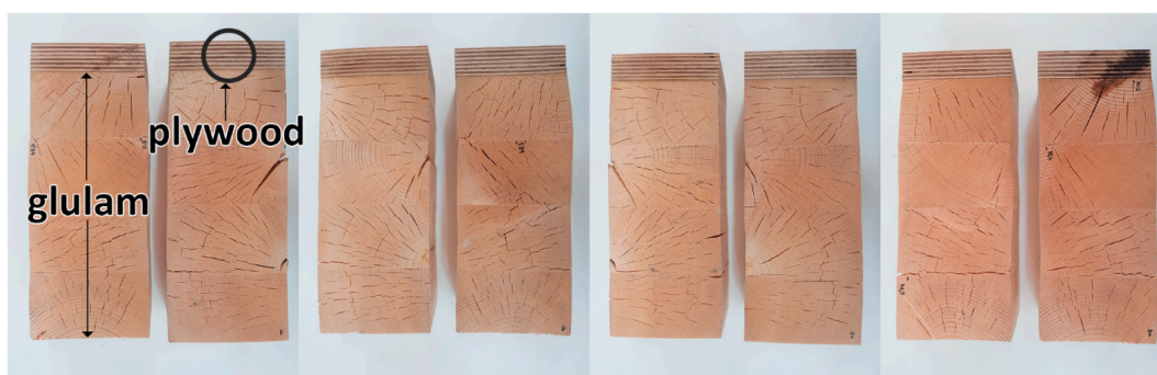
Fig. 12. Test pieces after the delamination tests.
