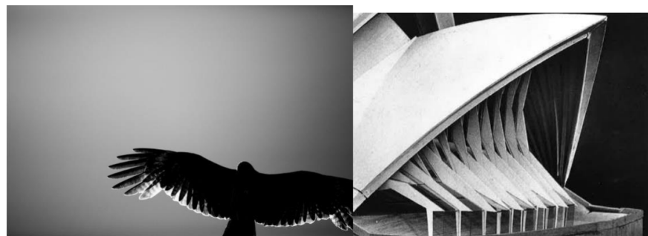
Figure 11. Left: image of a bird in flight, which Utzon used as a reference for the development of the facades ( https://pxhere.com/es/photo/1224384 ; last accessed 2 December 2021). Right: glass wall design principle (Yellow Book, 1962); ( www.records.nsw.gov.au ; last accessed 2 December 2021) [21].
