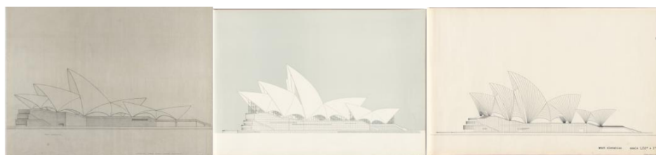
Figure 10. Design evolution. From left to right elevations drawing from 1956 (Brown Book, competition proposal), 1958 (Red Book, elliptical geometry), and 1962 (Yellow Book, spherical geometry) ( www.records.nsw.gov.au ; last accessed 2 December 2021) [21].
